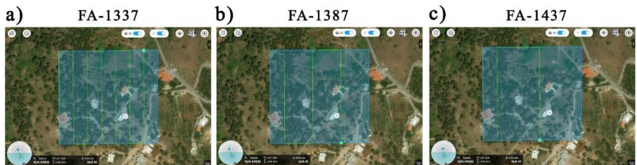
Fig.8.2. Flight paths are designed in the DJI ground control flight planning mobile application. The flight rectangle is approximately 196 x 180 m, representing a single flight sequence. a) flight path of 1337 m altitude, b) flight path of 1387 m altitude, c) flight path of 1437m altitude.
